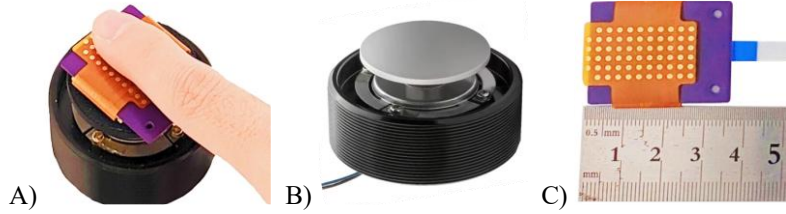
Fig. 1. Experimental Setup: (A) Overview, (B) Vibrotactile, (C) Electrotactile part.
